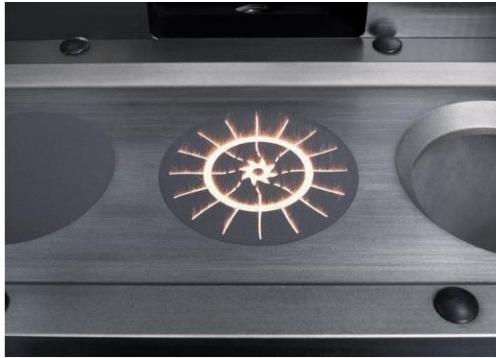
Figure 2 Laser metal fusion (LMF)[3]
